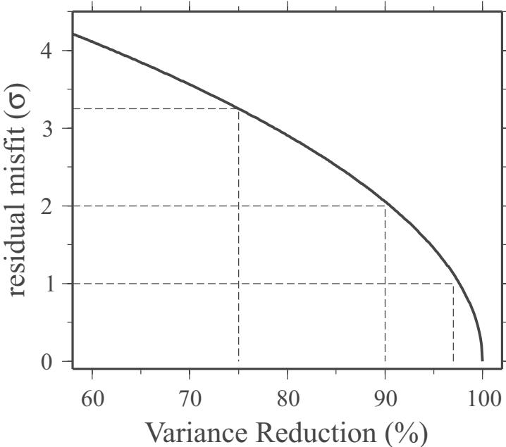
Fig. 2. Datafit metrics for proxy-CO<sub>2</sub> data. The total data variance is based on standard deviation  $\sigma$ , from the Pleistocene average (250 ppm). The variance of the 10-My moving-average proxy-CO<sub>2</sub> data corresponds to  $6.5\sigma$  rms misfit. Three approximate reference points are marked by dashed lines: 75% data variation and  $3.25\sigma$  data misfit, 90% data variance fit and  $2\sigma$  data misfit, and 97% data variation and  $1\sigma$  data misfit.
