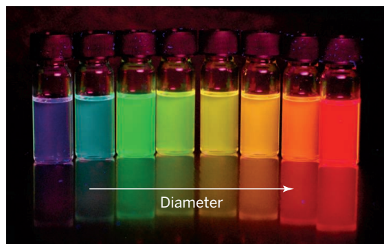
Color shift. Colloidal nanocrystals have size-dependent optical properties. For example, photoluminescence of CdSe nanocrystals shifts from blue to red with increasing diameter.
